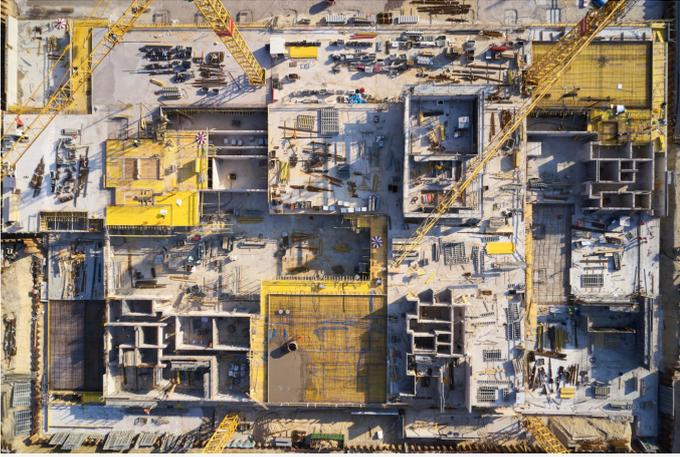
The first five-storey building, "The Pioneer", integrates three column-free halls spanned by steel girders. Modern workspaces will be created in 9,000 m<sup>2</sup> of office space above the production halls for approximately 600 technology specialists.
