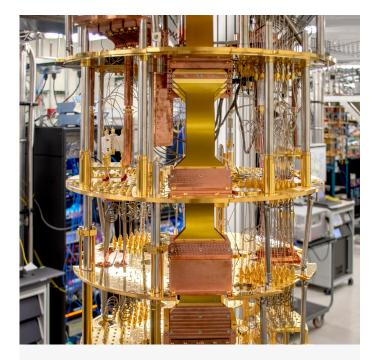
Detailed view of the IBM quantum computer. As of January 2023, QuantumBasel will have access to the IBM quantum computer with 433 qubits.
