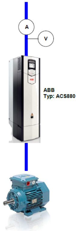
Synchronreluktanz-Motor IE4 Eff. 93.9% (15kW) + 94.2% (18.5kW)
